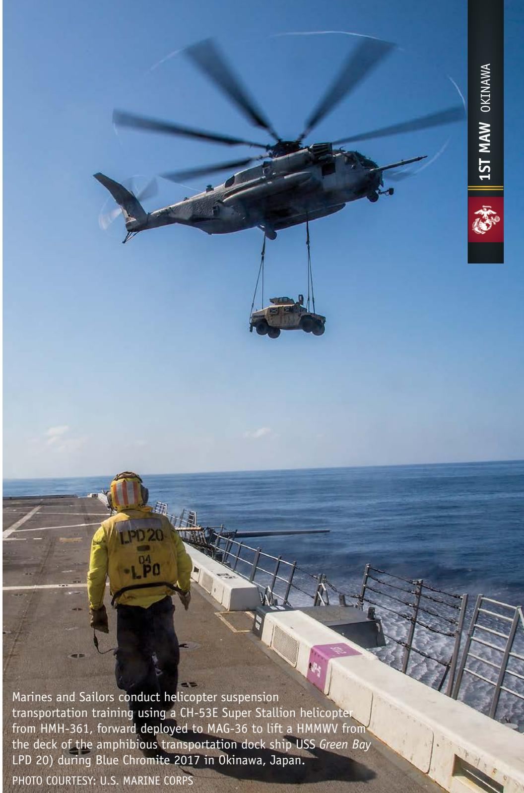
Marines and Sailors conduct helicopter suspension transportation training using a CH-53E Super Stallion helicopter from HMH-361, forward deployed to MAG-36 to lift a HMMWV from the deck of the amphibious transport dock ship USS Green Bay (LPD 20) during Blue Chromite 2017 in Okinawa, Japan.
